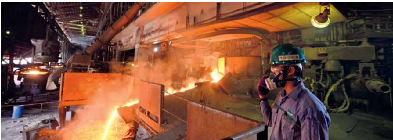
Proses Metal Tapping di Pabrik Feronikel Pomalaa Metal Tapping Process in Pomalaa Feronickel Plant
